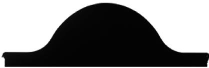
图 6 动态刀补条件下加工零件轮廓图像 Fig. 6 Image of workpiece profile with dynamic tool compensation
